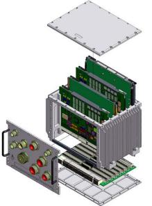
**Board Capacity** The E110 accommodates 6 standard VME boards with 0.8 inch pitch, including:
