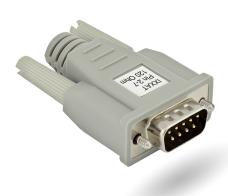
This connector provides easy and quick termination to any high-speed CAN or CAN FD product. The connector is used when a CAN node without internal termination needs to be terminated or if no CAN node is connected at the end of the CAN bus. According to ISO 11898-2, high-speed CAN buses / systems must be terminated at their ends by resistors.
