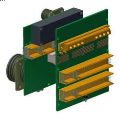
The customized backplane and the I/O transition board are designed using the same I/O signal characteristics, ensuring full matching of controlled impedances and signal integrity.
